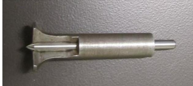
Center Punch Tool w/ Alignment Edges
