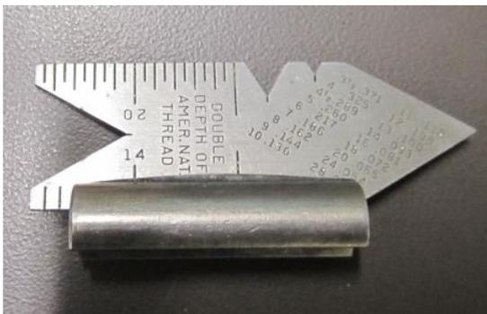
Fish Tail w/ Integral V-Cut Alignment Rod
