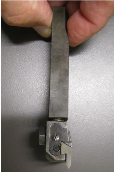
Thread Cutting Tool w/ Adjustable Lead Angle
