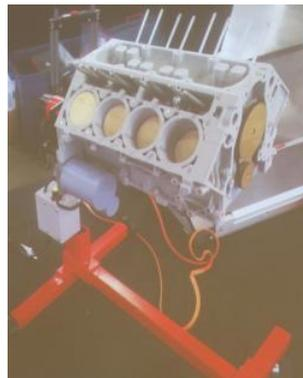
3D Printed Plastic V8 Engine
