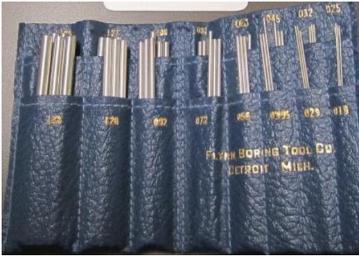
Thread Measuring Wires
