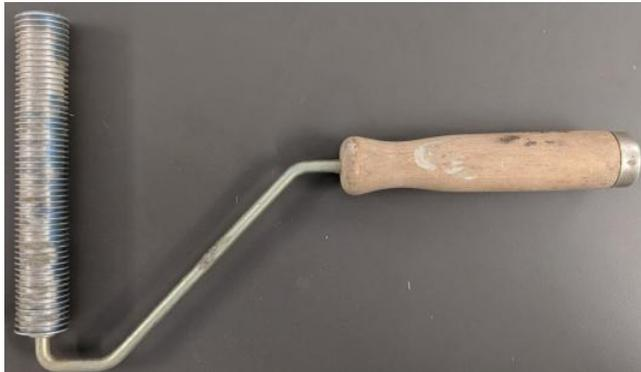
Special Roller for Eliminating Air Pockets
