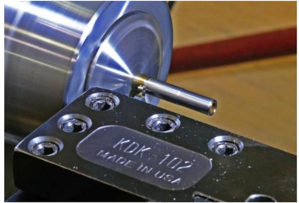
Assembly was completed by use of several Loctite Anaerobic adhesive products. He used 609 Retaining Compound for the blade to handle bonding and 242 Threadlocker to secure the sleeve in place. He used SF 7649 Primer on both locations since the bonds were between steel and aluminum and steel and stainless steel. Primer is not needed when bonding steel to steel.
