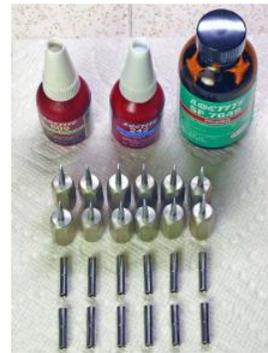
Final assembly by Loctite anaerobic: Aluminum & stainless need Loctite 7649 primer to cure adhesive.
