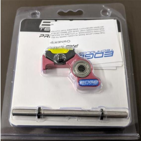
The rod, which comes with the gadget, would be mounted in the headstock. The flat would rest on the top of the cutting tool's cutting surface and then the tool height would be adjusted until the spirit level indicates a level position. This works since the bearing axis and flat are in the same plane. This, of course, presumes that your lathe has been leveled.
