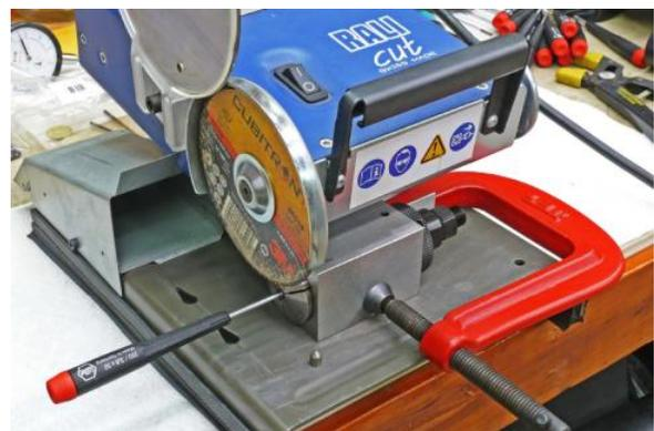
installed. The collet stop provided the repeatability from one cut to the next for the 12 screw drive blades he cut. This setup resulted in a total variation of length for all twelve blades of 0.0013". Not bad at all.
