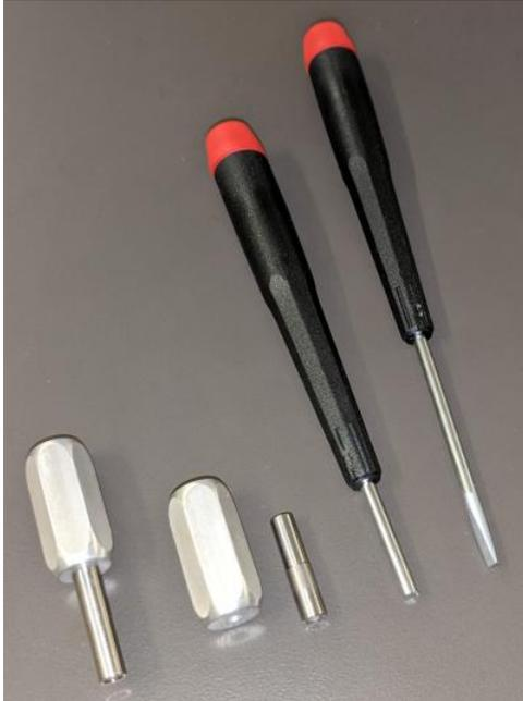
Making the knobs consisted of cutting sections of the 7/16" aluminum rod and then mounting them in a newly acquired 7/16" 5C collet for drilling and reaming to accept the screwdriver shafts. Also rounding sharp edges off using a form tool with a fixed radii.
