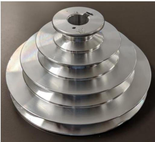
The only problem was there was no provision for a set screw(s) to keep the pulley in position on the shaft. Examining the pulley made it obvious why there was no screw. The only location where a set screw could be placed had a
