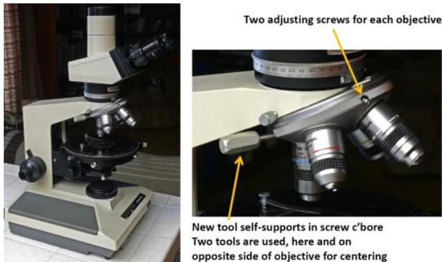
This is achieved by two adjustment screws and a spring, each separated by 120 degrees around the axis. The adjustment screws are a bit unique in that they allow the temporary mounting of adjustment screw drivers so that the two screws can be simultaneously adjusted without the need for a third hand. These special screw drivers are either no longer available or are prohibitively expensive, so Larry needed to come up with a replacement.
